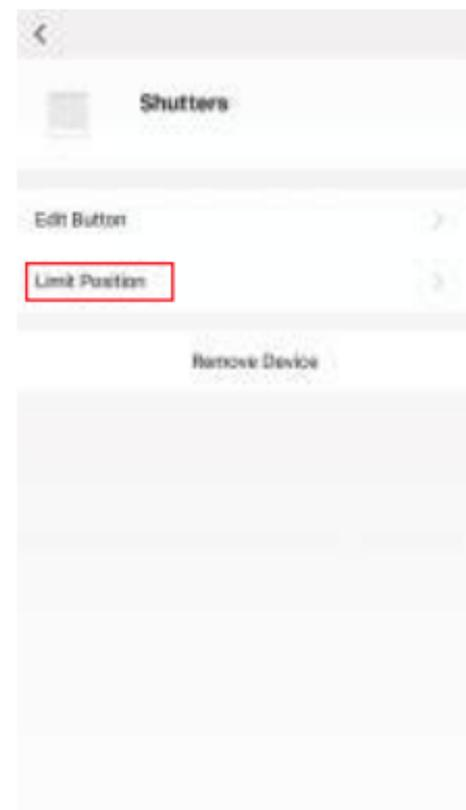
3. Choose "Up limit", tap "open" or "close" to the desired Up limit position, then "pause", tap "Save limit", the Up limit setting done. Motor runs downwards automatically, tap "pause" when it reaches the desired Lower limit position.
